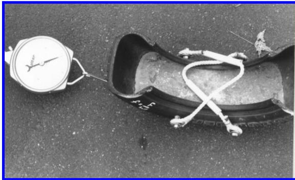
As the coefficient of friction is simply the horizontal drag force divided by the object's weight when the object is sliding across a surface, measurement systems utilising a dragged test tyre have been devised. A simple technique is to use part of a tyre filled with concrete dragged with a spring scale as shown below. The angle of pull is parallel to the surface.
