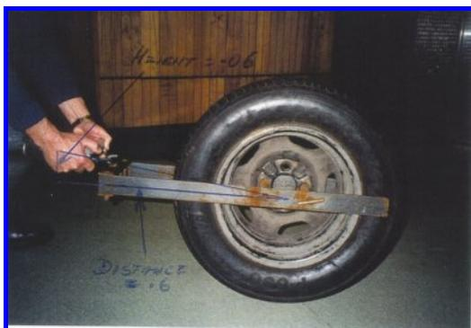
A clamp system can be used to create a drag wheel from the incident vehicle, as shown in photograph 5, and the same test methodology followed. While the drag wheel overcomes some of the alleged shortcomings of the drag sled/concrete filled part tyre, the problems of light load and needle fluctuation on the undamped spring scale remains.
