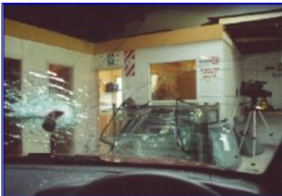
Laminated windscreens do not shatter or become opaque when broken. Adequate forward vision is retained. They also assist to retain occupants inside the vehicle when seat belts are not used. In this example a carpenter's hammer has penetrated the windscreen. Apart from localised damage around the impact area, the remainder of the screen provides acceptable vision.
