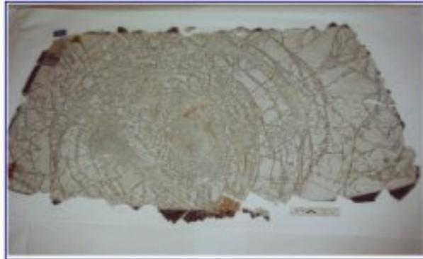
*Photograph 12 Reassembled laminated screen*
