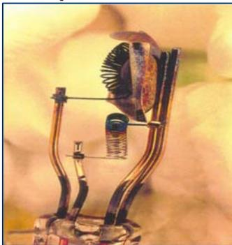
A careful inspection of the lamps will assist the investigator to determine if the lamp was ON or OFF. This will be of importance at night for opposing direction or intersection type crashes. In this example the driver was utilising dip beam when impact occurred and the quartz globe was shattered.
