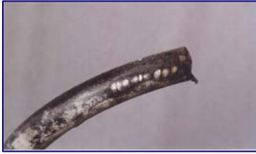
Some drivers carry out modifications to their vehicles. Inspection not infrequently reveals springs missing or brutally modified. These examples are of coil springs recovered from a vehicle post crash were modified with a hack-saw. In this case the driver was under the impression that the lowered, "sporty" look was the "in" image, claiming improved handling because of a lowered centre of mass. In each case control was lost while cornering and occupants died.
