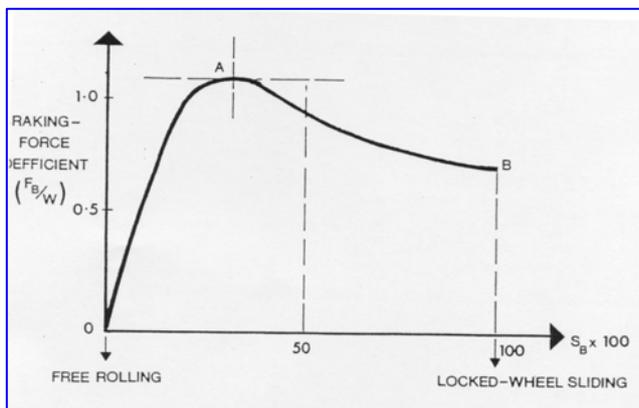
A common friction curve for a vehicle is similar to this chart. As the brakes are applied the force rapidly increases up to the point where the wheel locks. There is then a marked decrease in the braking effect, which when once past the initial lockup holds to an almost constant line.
