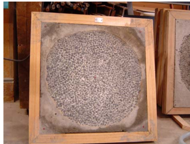
Figure 9: Hand placed Sample preparation Figure 10: Completed sample in timber frame
