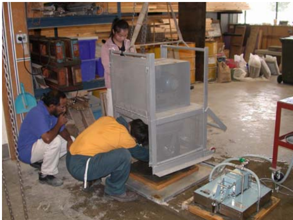
Figure 7: The UoA Accelerated Polishing Machine
