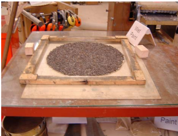
Figure 9: Hand placed Sample preparation Figure 10: Completed sample in timber frame
