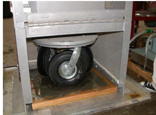
Figure 8: The Accelerated Polishing Machine wheel assembly unit in operation
