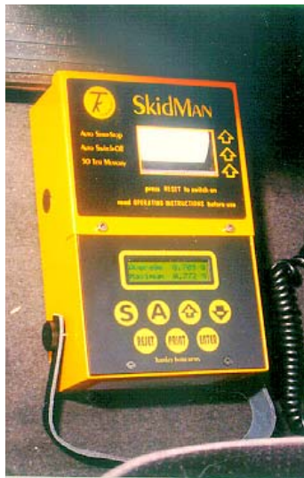
Figure 4a: Turnkey Instruments Skidman decelerometer used to estimate coefficient of friction ( \mu ) from the results of controlled skid tests using the collision vehicle or investigation vehicle (Photo from Turnkey Instrument Ltd)
