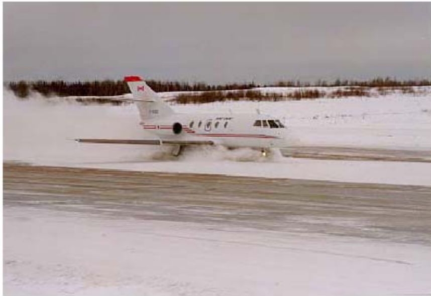
Figure 3. Photograph of Falcon-20 aircraft during test run on snow-covered runway.
