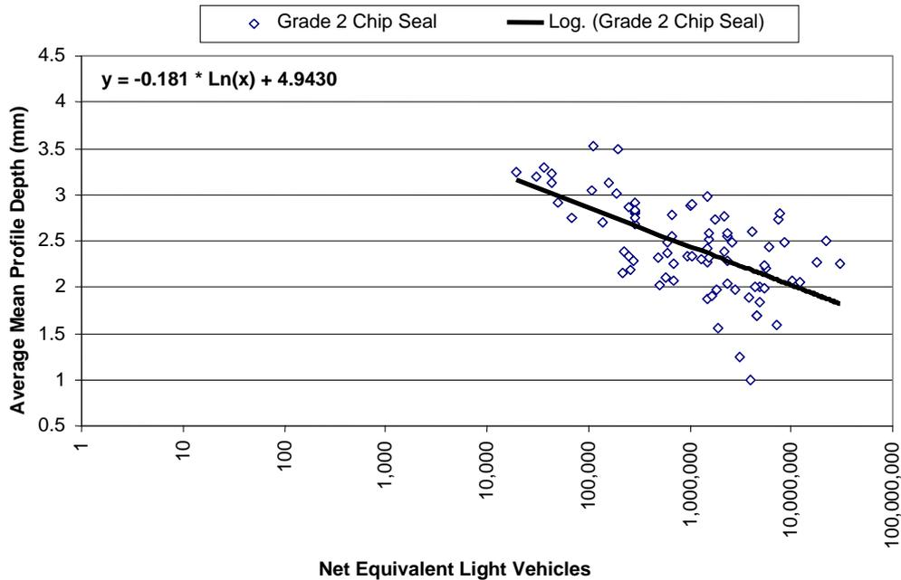
**Figure 4.3 – Method 3 Regional Calibration Principle (Grade 2 Chip Seal Example)**
