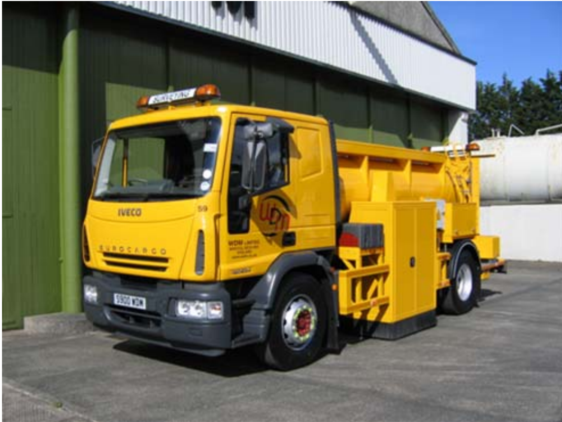
Figure 3: Sideway-force Coefficient Routine Investigation Machine (SCRIM).
