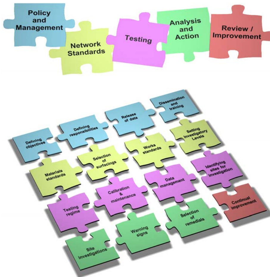
Figure 2: The sixteen key building blocks (and their five main headings) of a skid resistance management strategy from Austroads (2005), illustrated as jigsaw pieces
