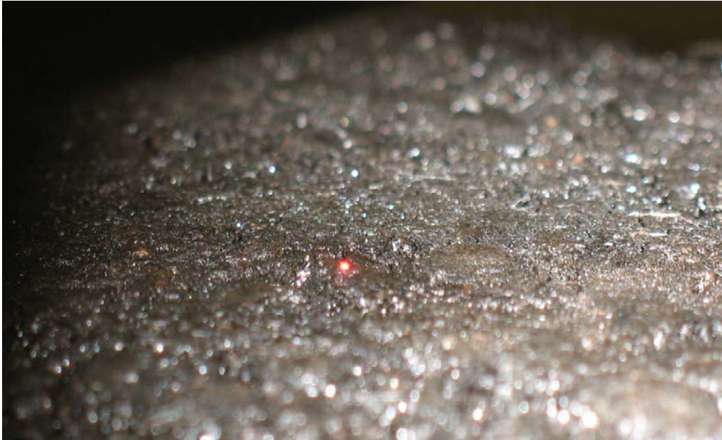
Figure 7: TM2 laser light on dense graded asphalt
