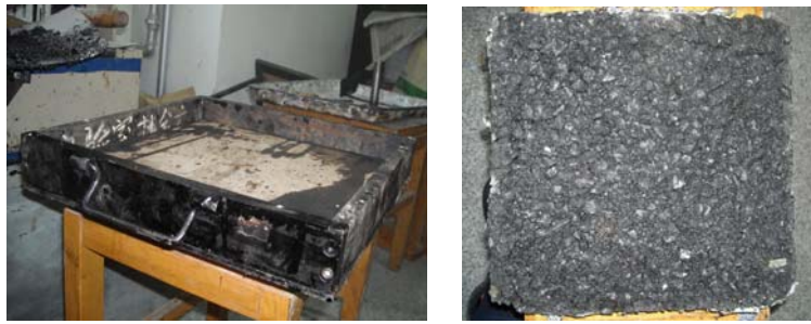
Figure 2: AC-13 filing block with 40mm thickness.
