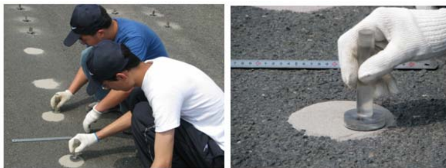
Figure 6: Texture depth tracking test.
