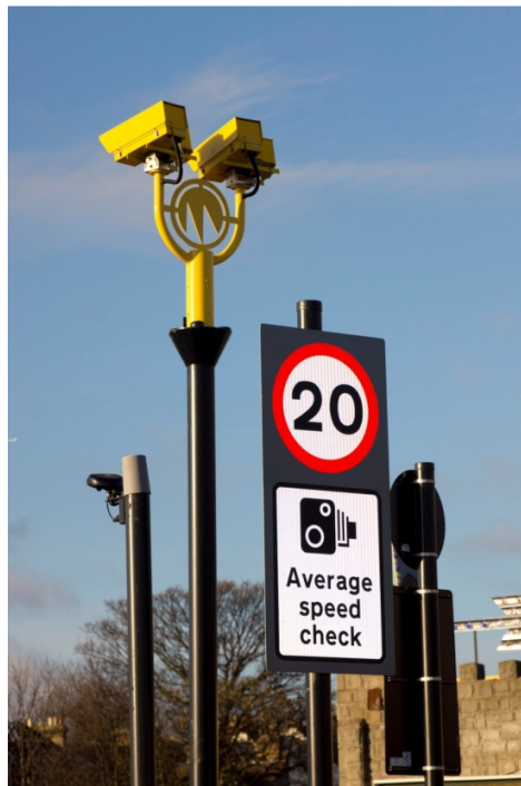
Figure 1: A SPECS3 POD installation in use on Marine Parade, Southend (Essex). This installation covers a 20mph limit along the sea front.
