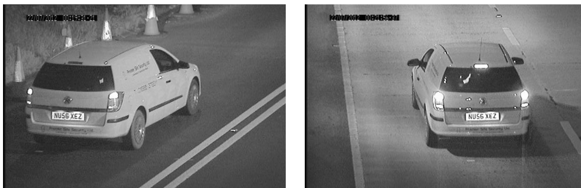
Figure 2: SPECS3 POD offence images, taken in complete darkness using infra-red overview illumination. This site is the A465 Head of the Valleys in South Wales.
