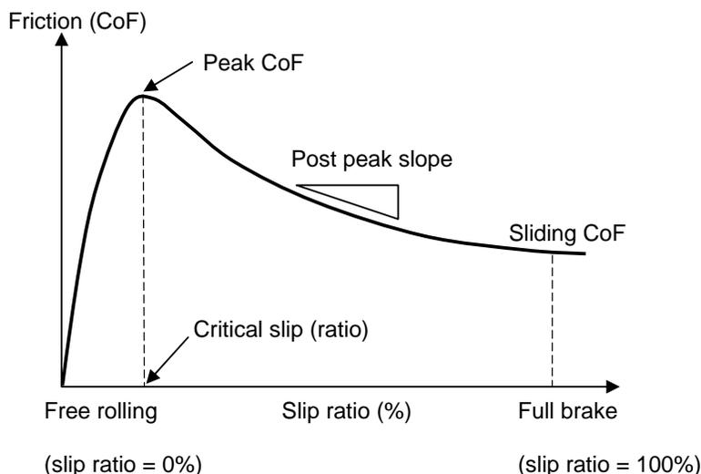
**Figure 2: Illustration of varying friction during a braking cycle**
