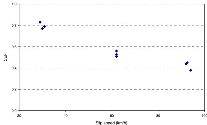
**Figure 3: CoF measured under different slip speeds**
