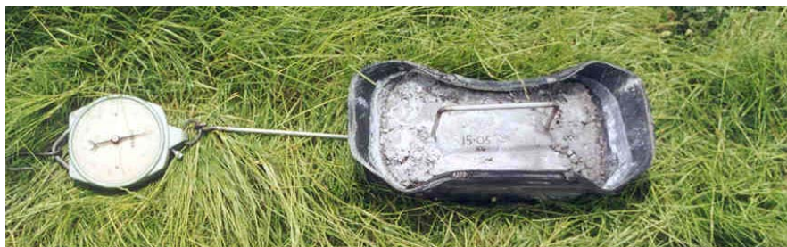
Figure 1: Tyre dragging test in progress
