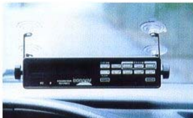
Figure 3: Vericom™ VC2000 unit mounted in test vehicle
