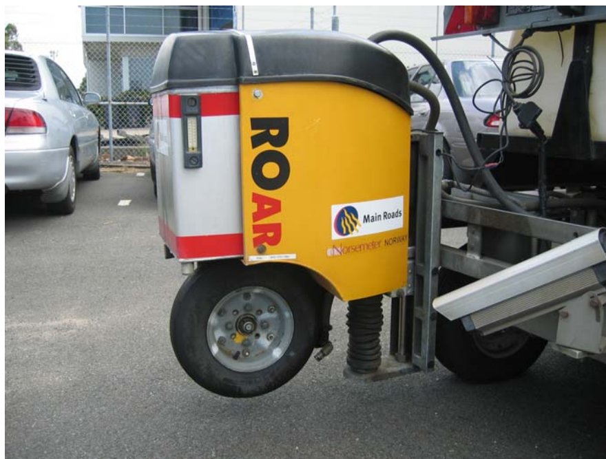
Figure 3: Norsemeter Road Analyser and Recorder or ROAR used by TMR (Baran, 2009)
