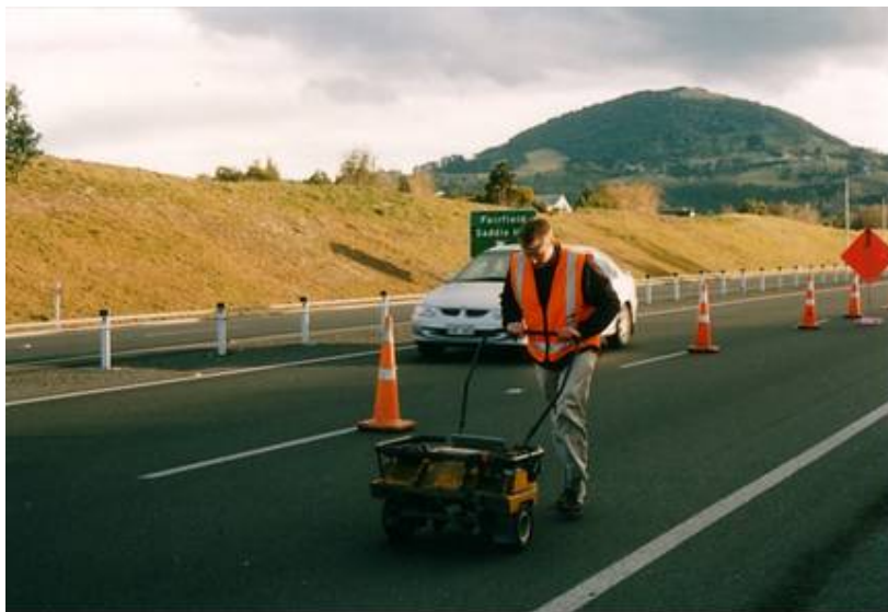
Figure 4: GripTester being used in push mode
