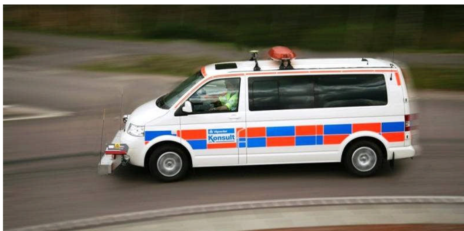
Figure 7 SRA CS's laser/inertial Profilograph P45 [Photo: Mats Landerberg]
