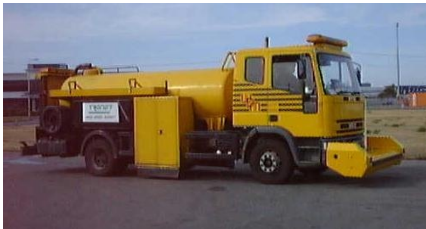
Figure 2: The first SCRIM+ 1998/9: scrim + high speed survey vehicle.
