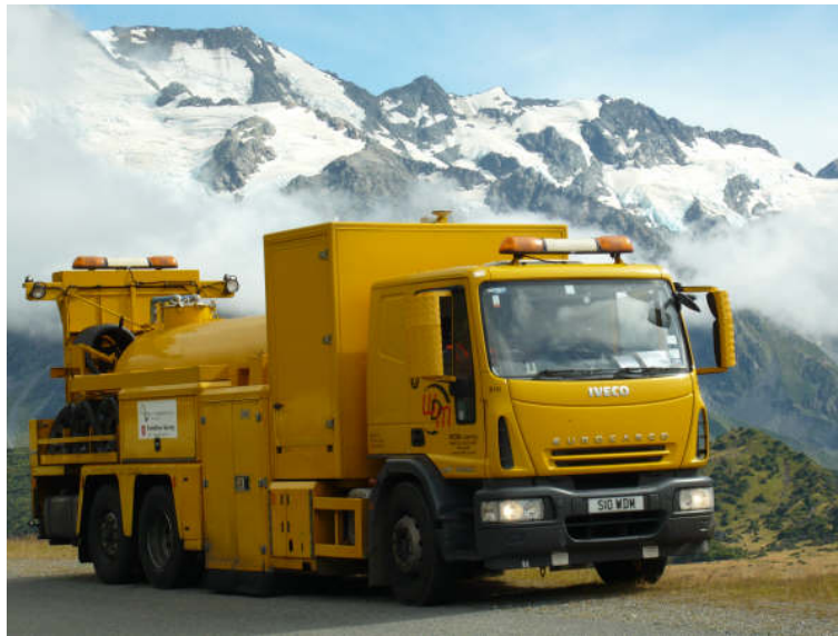
Figure 4: The third SCRIM+ 2007/2008: SCRIM + high speed survey vehicle.
