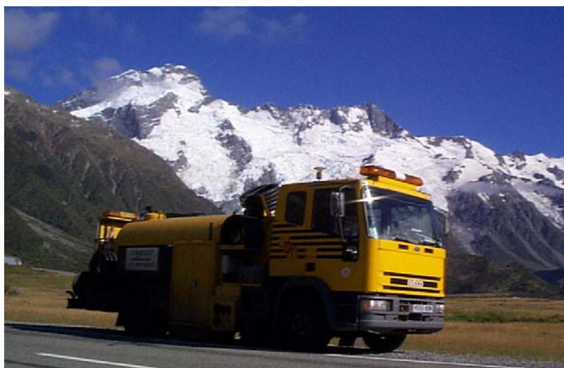
Figure 3: The second SCRIM+ 1999/2000: scrim + high speed survey vehicle.
