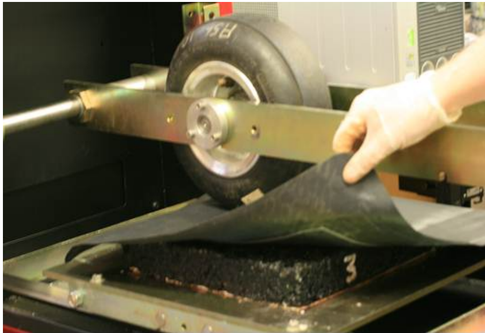
Figure 6: Modified Wessex wheeltracker test rig with slab and pressure mat
