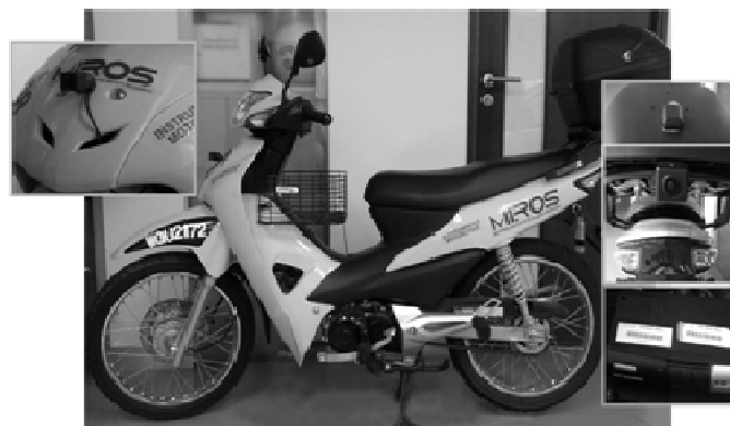
Figure 1. The instrumented motorcycle used in the study
