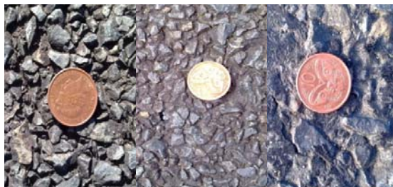
Figure 4: Photographs of Good (Left), Medium (Middle), and Poor (Right) Macrotexture.
