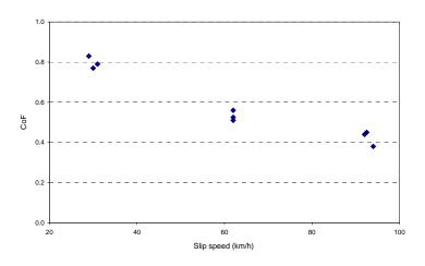
Figure 3: CoF measured under different slip speeds
