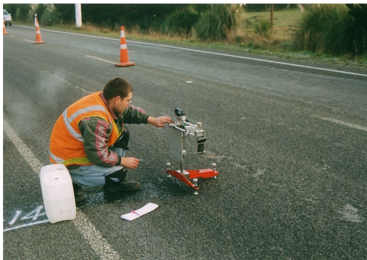
Figure 3: The British Pendulum Tester on Coarse Chipseal
