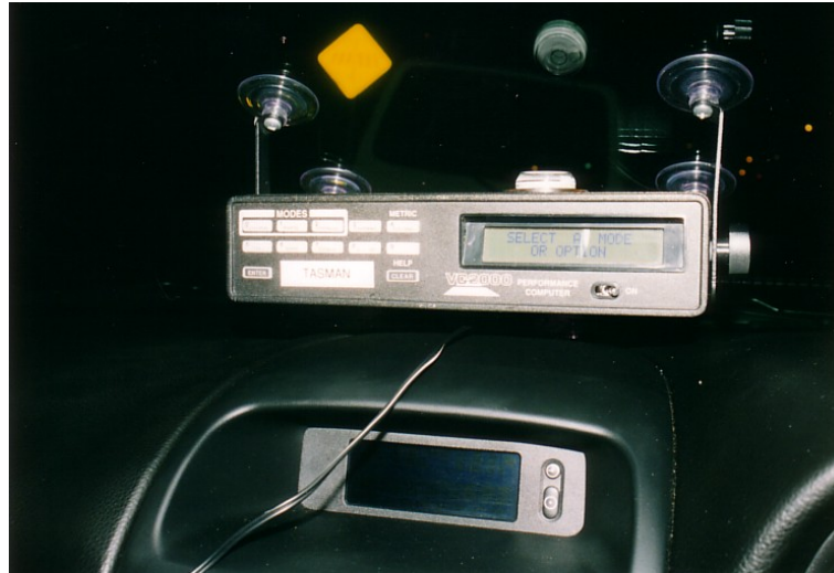
Figure 4: Vericom VC2000 unit mounted on the windshield of the test vehicle
