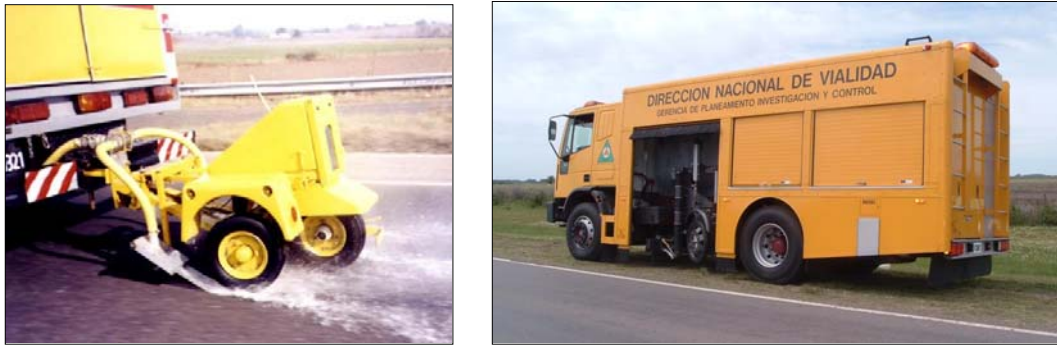
Figure 2: Mu meter and Scrim Tex used for National Road Administration in Argentina.
