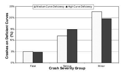
Figure 4-4: Crash severity per Curve Deficiency
