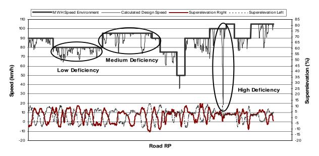
Figure 3-2: Curve Deficiency Plot
