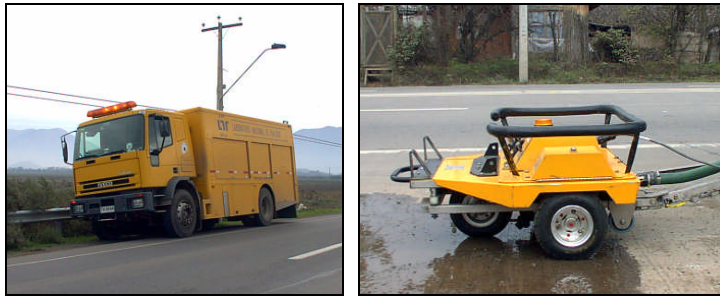
Figure 2. SCRIM and Grip Tester devices used to measure skid resistance in Chile (Source: Tomas Echaveguren with permission of NHL).
