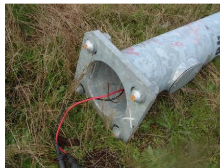
Couplings sheared and the light Pole was not damaged.
