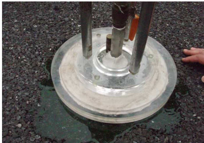
Figure 10: Incomplete watertightness of water sealer
