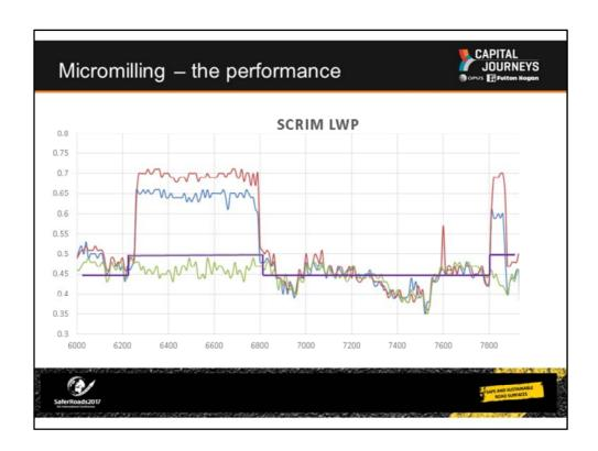
The next test, in May 2016, 4 months after treatment, shows the initial rapid polishing of the aggregate, on both of the test sites milled, of note the large site was the OGPA 20, the smaller on a OGPA 10, in terms od SCRIM, performing equally.
