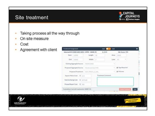
Again following desktop analysis, the data is taken into the field with the FIT. With the GPS enabled, the treatments can be reviewed, site markup completed, and recorded for upload along with photographic site records. Additional functionally now built in records the cost of the treatment in line with the approved schedule, giving up to date visibility of budget allocation and remaining funds.
