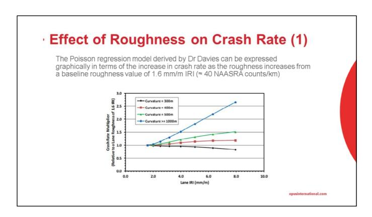
Figure shows, for example, that for roads with a horizontal curvature of radius greater than or equal to 1000m, a 40% reduction in the IRI roughness from 5mm/m to 3mm/m will result in a reduction in the crash rate of about 28%. However, if the horizontal curvature is tightened to 400m, this 40% reduction in road surface roughness will result in a reduction in the crash rate of only 8%.
