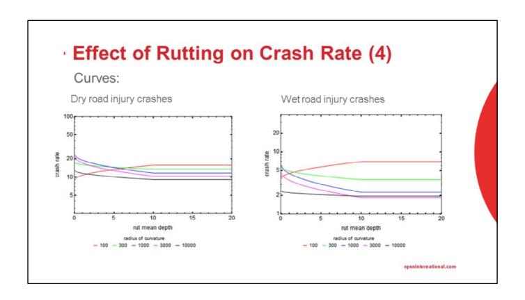
The crash rate reduces as rut depth increases for curves with a radius of curvature in the range 1000m to 3000m. The effect is weaker for curves outside this range. The graphs suggest that crash rates increase with rut depth for very curved roads, but this might be partly due to the way the predictor variables are defined.
