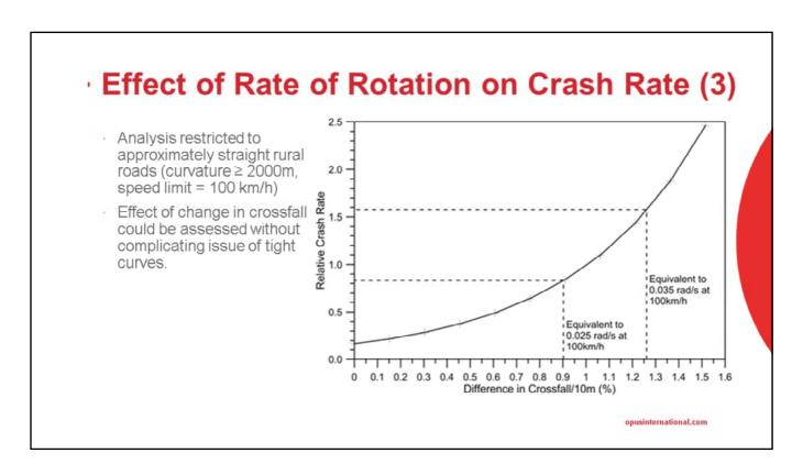
This analysis showed that changes in crossfall, and hence the rate-of-rotation, do have a statistically significant effect on the crash rate. The relationship is shown in the plot. This shows the relative change in crash rate against the change in crossfall for each 10 m road section. Also shown on the plot are the changes in crossfall that correspond to the  $0.025 \, \text{rad/s}$  and  $0.035 \, \text{rad/s}$  threshold limits<sub>7</sub> for a vehicle travelling at  $100 \, \text{km/h}$ .
