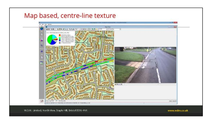
Using public available mapping, together with WDM software running on a server gives a client access to the information, and, using client defined criteria, enables the data to be presented against map backgrounds. The video images collected during the survey can be shown and shown linked with the data presentation.
