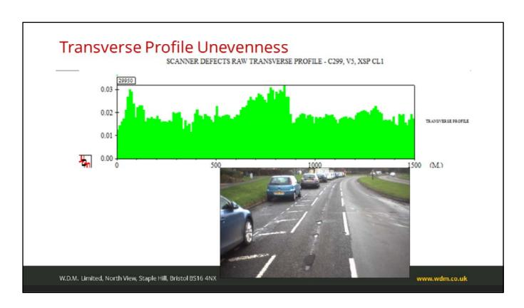
Data can be reported in tabular form and plotted a results over a given length of cycleway. This show the measure of transverse profile over a 1,500 m length with an image associated with the high values near the centre of the length.
