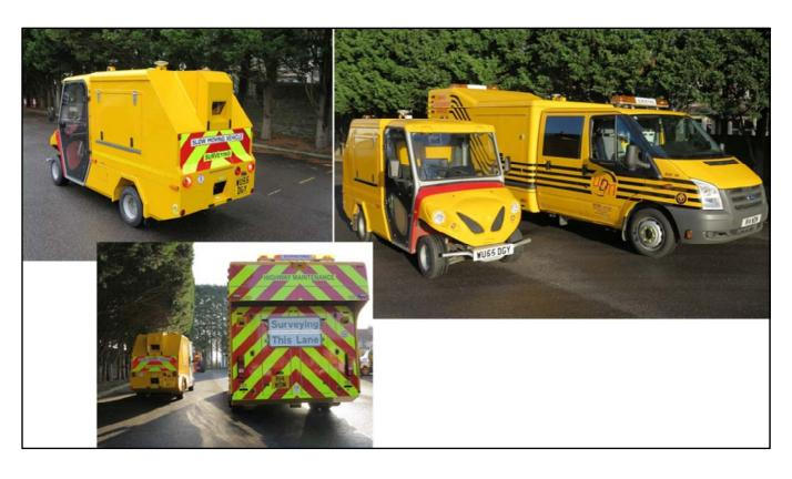
Size chosen to reflect the narrow nature of cycle ways This shows comparison with one of our conventional high speed data collection vehicles or Road Assessment Vehicles, RAV's.
