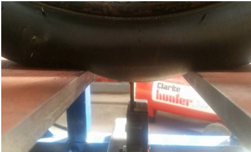
Figure 5. Sideways force tire deforming into the space between plates.
